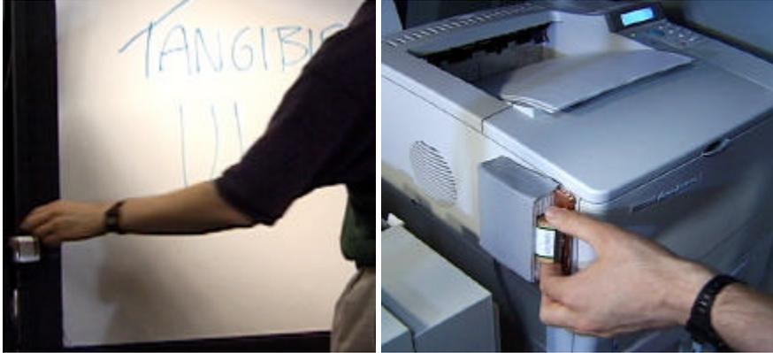
**Figure 4.2: Whiteboard, printer mediaBlock slots**
